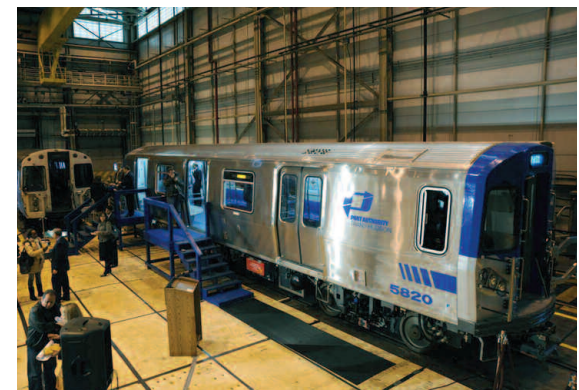
The new PATH cars will feature three doors on each side to allow faster loading and unloading.
